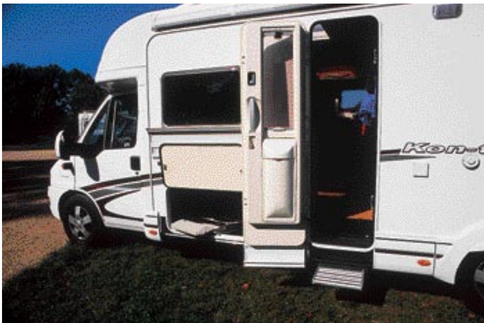
A new caravan door adorns the 660, complete with two-point locking, waste bin and window. Forward of this is the access flap to capacious underfloor storage space.
