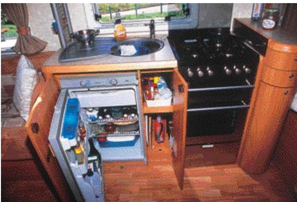
Slot-in cooker, AES fridge and removable drainer help make the 660's galley good to use.
